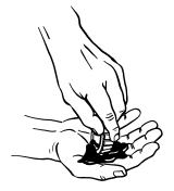
Lube Point(s) - Repack Capacity - A/R Lube - MPG Interval - Every 2 years or 1200 hours of operation
