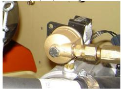
Interval - 3 Months or 150 hours of operation Comments - Replace filter. Refer to Section 6.6, Propane Fuel Filter Replacement
