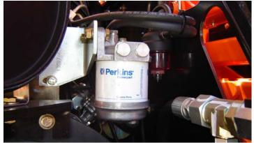
Lube Point(s) - Replaceable Element Interval - Every Year or 600 hours of operation 19. Air Filter
