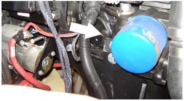
Lube Point(s) - Fill Cap/Spin-on Element (JLG P/N 7027965) Capacity - 4.5 qt. (4.25 L) w/filter Lube - EO Interval - 3 Months or 150 hours of operation Comments - Check level daily/Change in accordance with engine manual. 13. Oil Change w/Filter - Perkins
