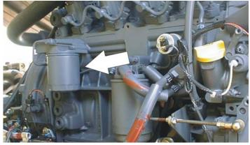
Fill Cap/Spin-on Element (JLG P/N 7016641)
